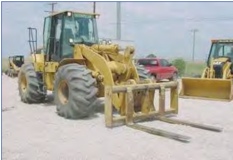
Front Loader w/forks to move sea containers
